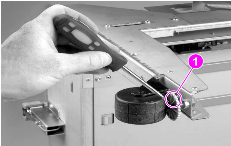
**Figure 159.** Removing the adjustable caster
