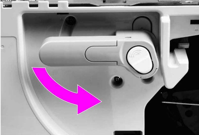
**Figure 69.** Removing the cartridge release lever (1 of 2)
